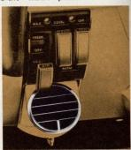
Cooled air is directed throughout the vehicle through two registers located in the instrument panel and two round registers one at each end of the panel. Air distribution from the center registers is controlled by louvers which are adjusted by a control wheel located in the center of each group of louvers. Pressing the wheel down deflects the air down-
