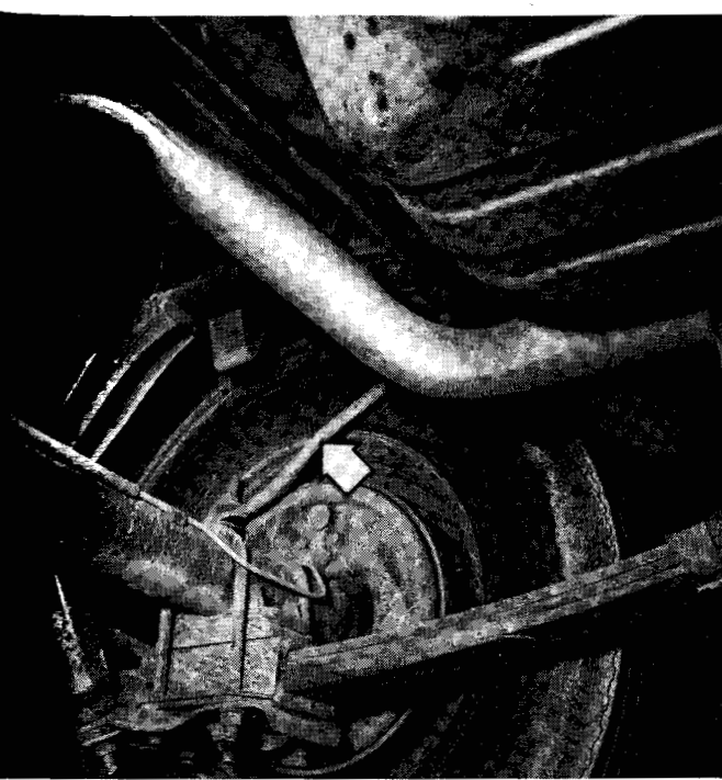
SPINDLY rear anti-roll bar, arrow, reduces the car's basic understeer to manageable proportions. A good buy.
