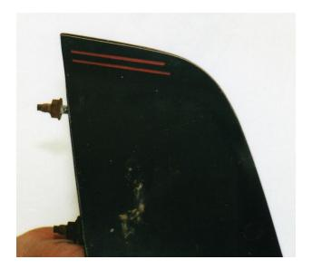
It is hard to give you a definitive size on where these stripes end on the front fender extension and rear quarter extension, because of the curve built in to these extensions. The figures I have are .275 for the top stripe on the front fender extension, and .600 for the top stripe on the rear quarter extension, again with the bottom stripe being slightly longer.
