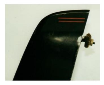
The top edge of the top stripe was .450 down from the top of the body line. As previously mentioned, on 68's there was a half inch gap at the 4 seams (front and rear of door, quarter extension, fender extension). On 67's the stripes are continuous through the seams.
