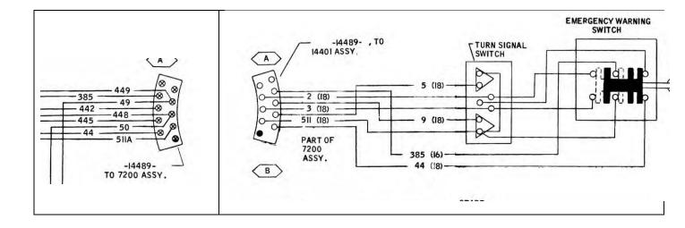
The table below follows the circuit diagram from top to bottom on the vehicle harness side from the outer row of pins starting with circuit 385 to 44 then top to bottom for the inner row of pins starting with circuit 449 to 511A. Note that circuits 449 and 49 on the vehicle side connect to the same circuit 2 on the switch side. Likewise circuits 448 and 50 on the vehicle side connect to the same circuit 3 on the switch side.
